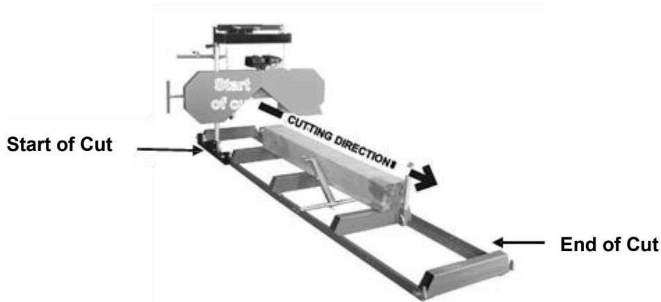
Figure V: Direction of Cut
